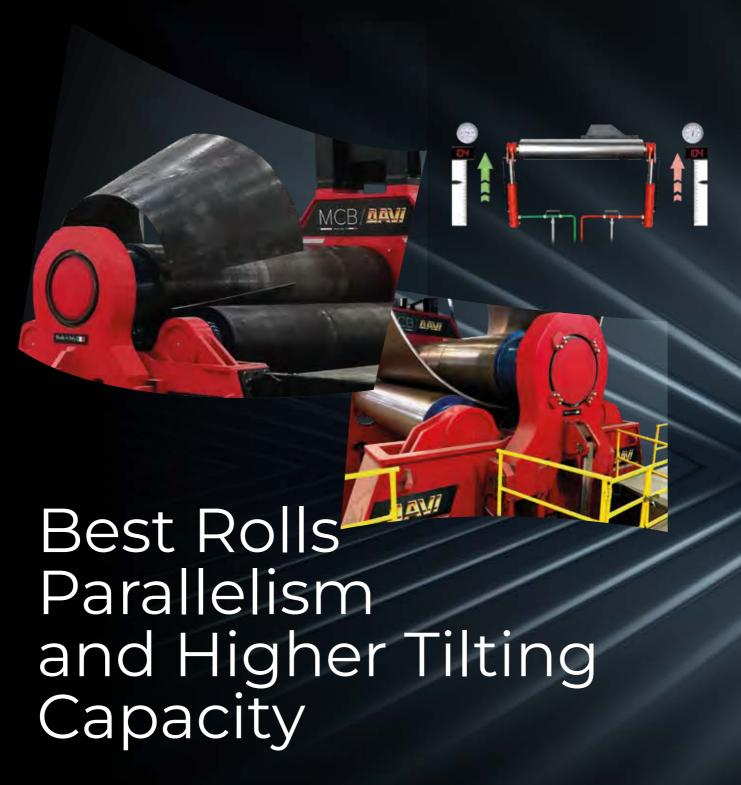
The patented Servo-Tronic® system keeps the machine's rolls parallel at all times thanks to its dual, independent but integrated, parallelism control system. This system features dedicated pumping groups and circuits guaranteeing that each cylinder receives oil at the very same pressure and mass flow, with electro-valves for fine-tuning only.
